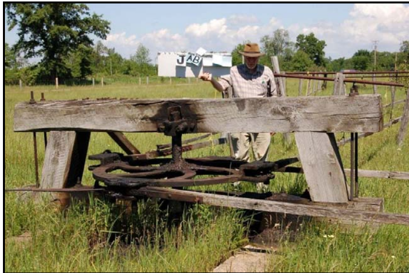
Figure B-8: Field wheel J-AB on James Field to divert the line 90°
