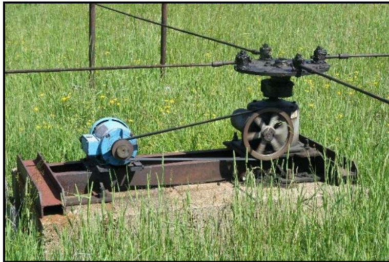
Figure C-3: Field motor on steel frame with steel jerker rods on the James Field
