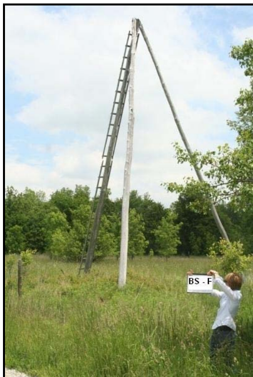
Figure C-2: Last standing original 3-pole derrick in the Oil Springs oil field, located on the South Byers field.
