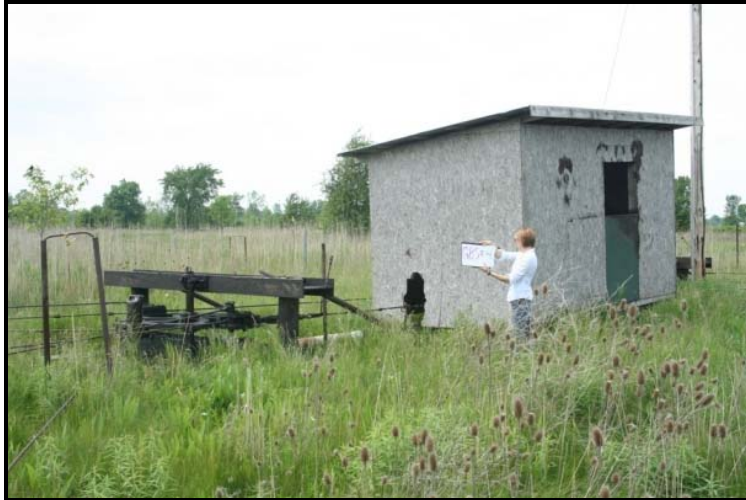
Figure B-13: Hybrid system of geared, enclosed electric motor with a Canadian system bull wheel.
