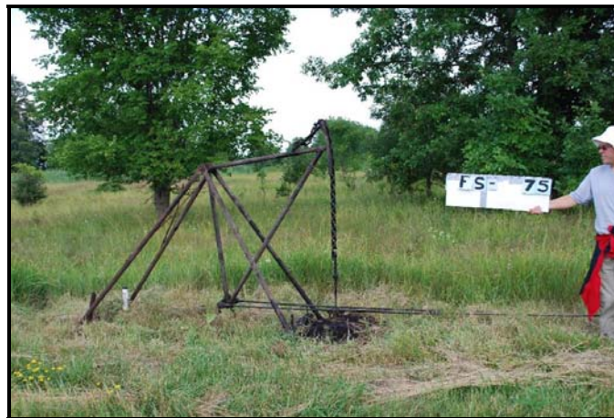
Figure B-11: Feature FS-75 Jones and Hammond pump jack on steel cable jerker line
