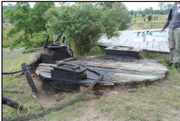
Figure B-19: Feature FS-AG, large wooden tank in background used for brine disposal system
